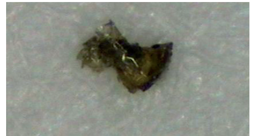
Fig. 35: Non-metallic particle, probably pink polystyrene packaging material
