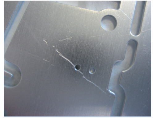
Fig. 67: Damaged metallic stiffener
