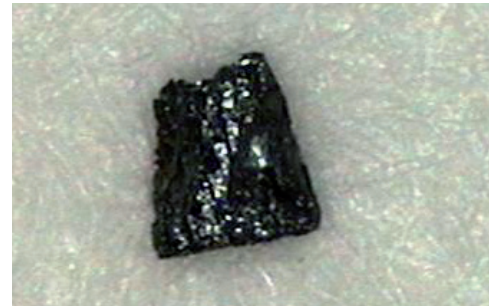
Fig. 33: Ferrite particle, identified as non-metallic (558 \mu\text{m} )
