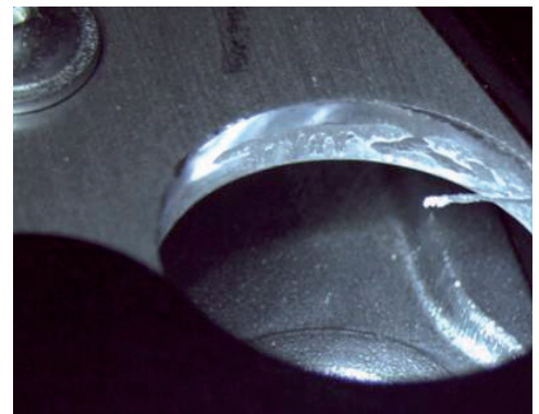
Fig. 69: Stamping residue loosened by pickling bath
