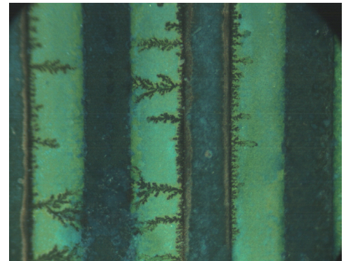
Fig. 104: Dendritic growth between the gaps of a comb-patterned circuit board
