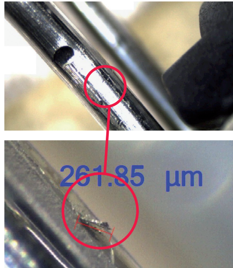
Fig. 27: Enlarged photo depicting particle length measurement
