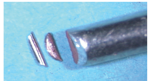
Fig. 24,25: Particles generated by wire cutting D = 1.8 mm (tinned copper)
