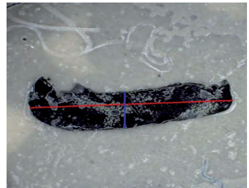
Fig. 71: Particles on externally supplied plastic elements
