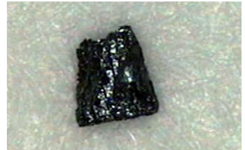
Fig. 33: Ferrite particle, identified as non-metallic (558 \mu\text{m} )
