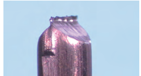
Fig. 23: Burr formation on copper wire (D = 2.25 mm) after use of wire-cutter
