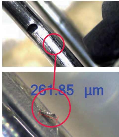
Fig. 27: Enlarged photo depicting particle length measurement
