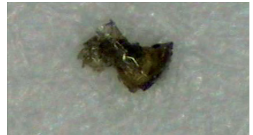
Fig. 35: Non-metallic particle, probably pink polystyrene packaging material
