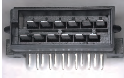
Fig. 52, 53: 12-pin connector with bridged contacts
