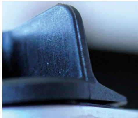
Fig.70: Plastic element with burr
