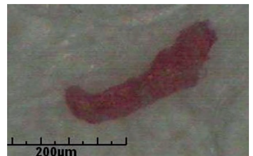
Fig. 35: Non-metallic particle, probably pink polystyrene packaging material
