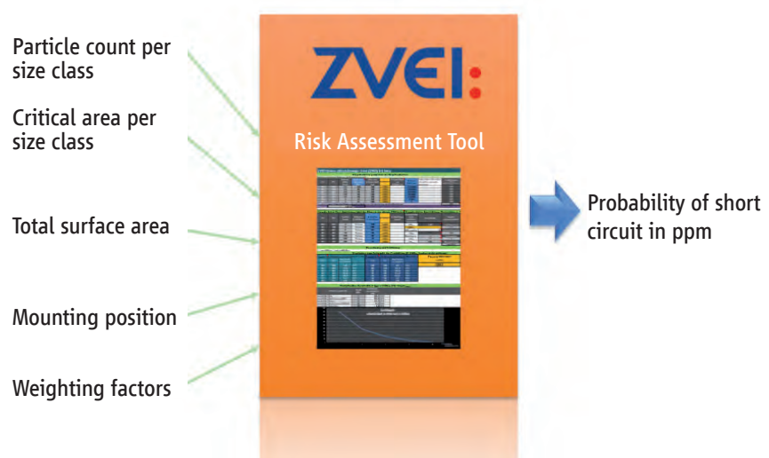
Fig. 95: Functional structure of risk assessment tool
