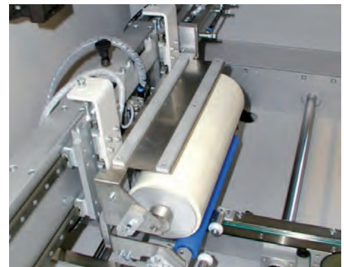
Fig. 86: Adhesive roller system for PCB contact cleaning
