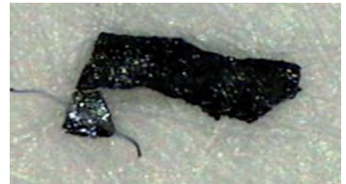
Fig. 34: Non-metallic particle, probably burr or plastic residue (217 \mu\text{m} )
