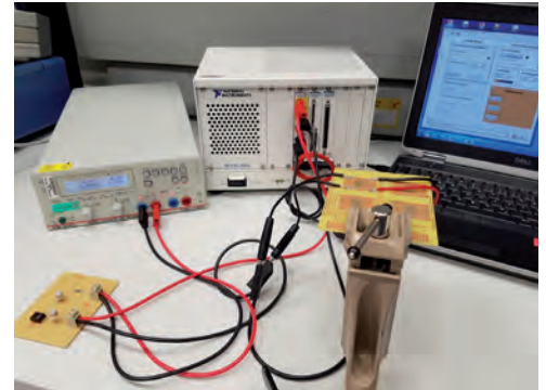
Fig. 92: Automated current measurement with software
